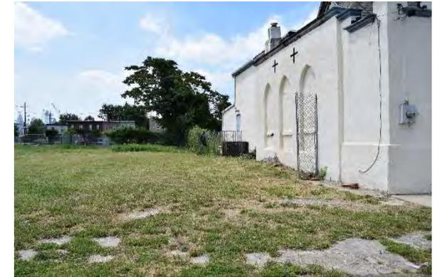
There are multiple downspouts around the church that can be redirected to the south side of the church where a rain garden can be installed to capture, treat, and infiltrate rooftop runoff. A preliminary soil assessment suggests that more soil testing would be required before determining the soil's suitability for green infrastructure.
