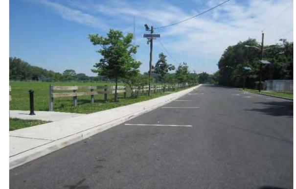
Stormwater currently drains to catch basins on the park road. A rain garden can be placed in the large grassed area to capture, treat, and infiltrate runoff from the roadway before it reaches a catch basin. A second rain garden can be placed behind one of the park buildings to capture runoff from the rooftop. A preliminary soil assessment suggests that more soil testing would be required before determining the soil's suitability for green infrastructure.
