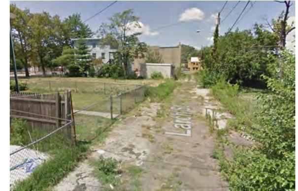
This alley on Larch Street is severely deteriorated, and a rain garden could be implemented to capture runoff from the pavement. As a potential alternative, the alley could be redone with turfstone or another permeable surface that supports vehicular traffic to repair the dilapidated pavement into a permeable surface. A preliminary soil assessment suggests that more soil testing would be required before determining the soil's suitability for green infrastructure.
