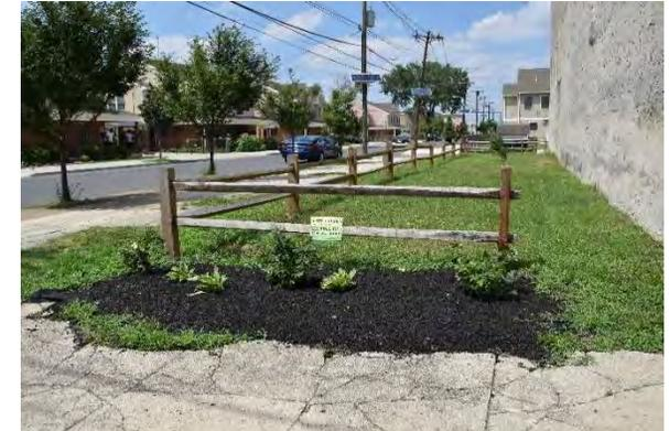
At the church, an existing area west of the church can be enhanced with a rain garden that could capture runoff from the roadway. An existing downspout at the front of the building can be redirected into a rain garden toward the rear area of the parking. A preliminary soil assessment suggests that more soil testing would be required before determining the soil's suitability for green infrastructure.
